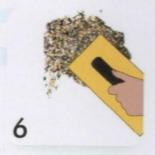
Applying liquid wallpaper to the prepared surface is made with a plastic trowel.
